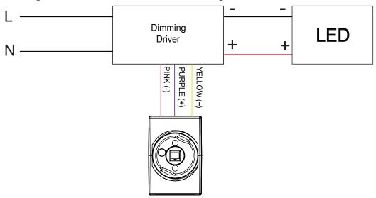
Wiring for AC/DC Adapter with dimming ballast or led driver.
